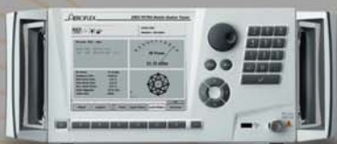
2303 STABLOCK TETRA MOBILE STATION TESTER
